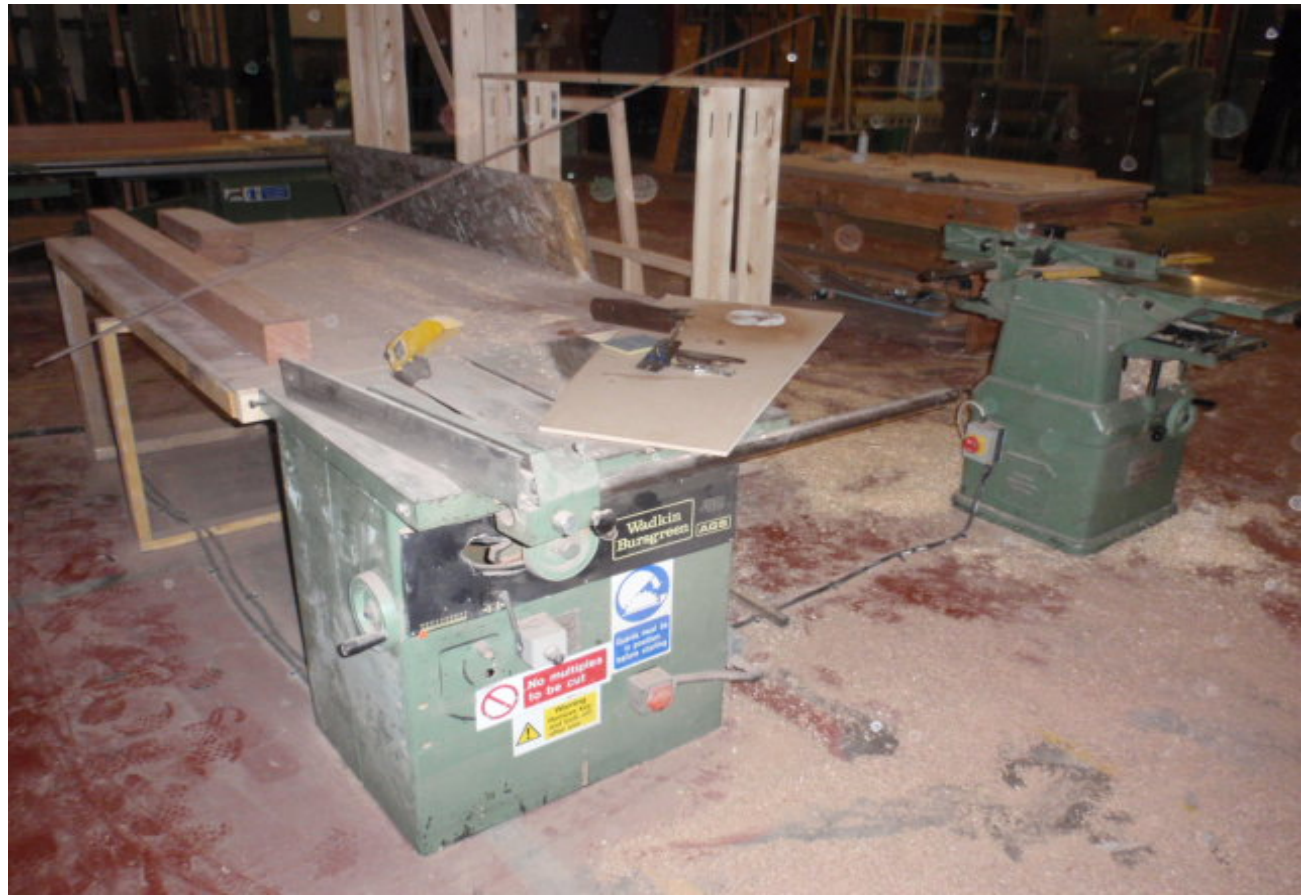
Sawdust spillage around a rip saw & planer
